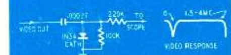
Fig. 10—Crystal probe for picking up the video output. At right is a video response as it should look on a scope.
